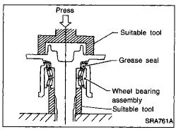
Press axle shaft into inner race of wheel bearing. Maximum load P:
