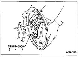
10. Position axle shafts in rear axle housing with Tool as a guide. Be careful not to damage oil seal.
