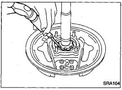
7. Unbend lock washer with a screwdriver.
