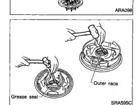
10. Remove grease seal in bearing cage with suitable bar.
