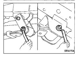
Tighten spring shackle nuts, front pin nuts and shock absorber nuts.
