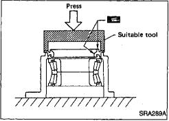
Press new grease seal until it bottoms end face of bearing cage.
